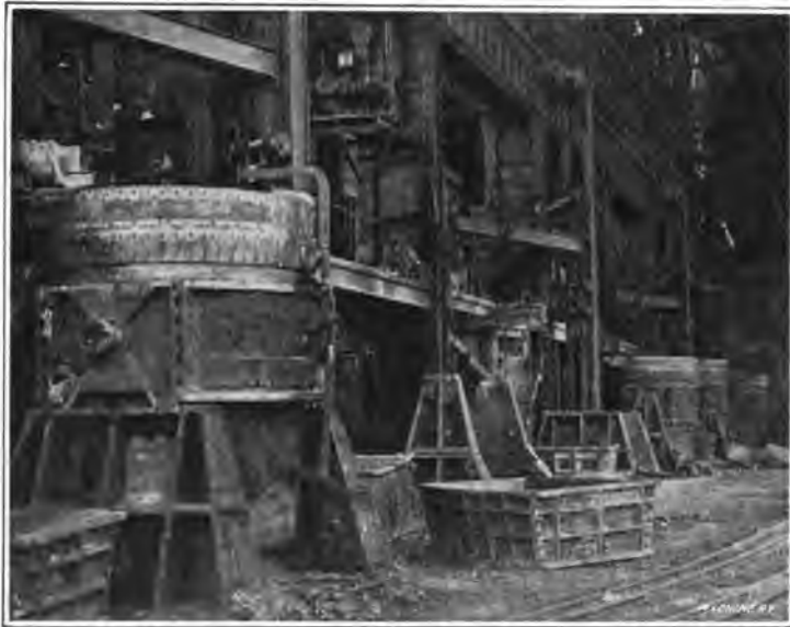
Fig. 4. Seventy-five-ton Ladles placed at Open-hearth Furnaces to Receive the "Heat" of Molten Steel—Homestead Works of Carnegie Steel Co.
